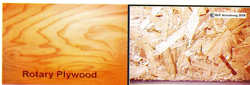
Figure 8: Specimen of a veneer produced by a rotary peeler
